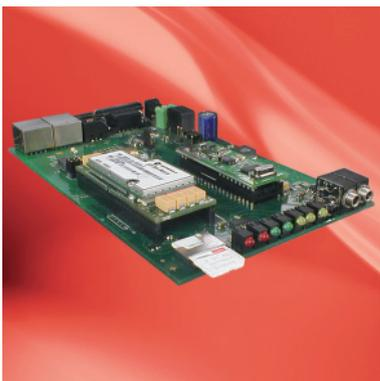
**XM-STK** Evaluation Kit for the socket modem family including all necessary cables, antenna and power supply.
